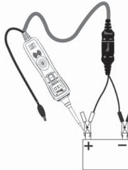
While the PP3 is in Power Probe Mode, contact the probe tip to a **POSITIVE** circuit. The red positive sign “+” LED will light and the voltage reading of the circuit will be indicated on the LCD display. If the audio feature is turned on, a high pitched tone will sound.
