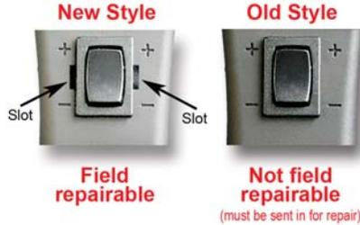
Remove the worn switch with a pry tool - be careful when applying force.
