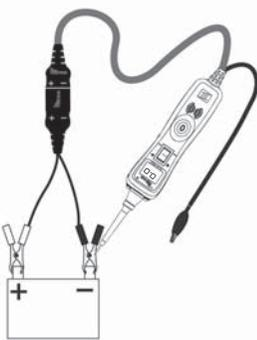
While the PP3 is in Power Probe Mode. Contact the probe tip to a **NEGATIVE** circuit. The green negative sign “-” LED will light. If the audio feature is turned on, a low pitched tone will sound.
