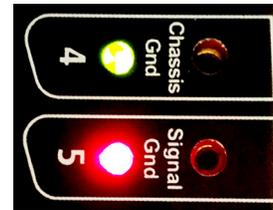
When the OBD-II Break Out Box is plugged into the vehicle DLC and detects reverse polarity in pin 4 and 5, the LED will turn RED.
