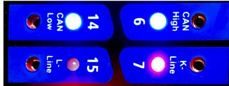
Depending on the communication protocols (Pin 6: CAN H, Pin 14: CAN L), Pin 2: Bus + Line), (Pin 10: PWM-), (Pin 7: ISO-9141
