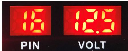
Default Pin display is always set to pin 16 with corresponding battery voltage display on its voltmeter (example: 12.5V) detected from the DLC.
